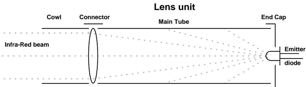
On its own an emitter diode produces a beam of infra-red light which spreads out by anything from 10 to 60 degrees or more as it moves away from the source. This is normally only enough for a range of about 20 to 30 meters.
