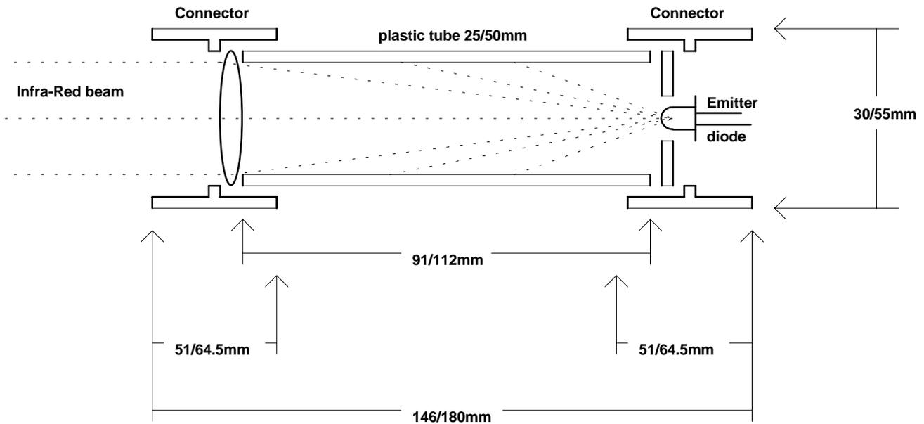
Two different sizes of SmartGun Lens Units are available, but general construction of both is the same as can be seen in the above diagram. In the measurements, the first size number is for the smaller unit. The lens unit is supplied complete ready-assembled with lens and emitter fitted.
